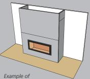
box wall installation, all made with SKAMOTEC 225.
